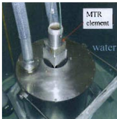
(c) AEFC System inside the water with MTR Fuel assembly from previous experiment [19]
